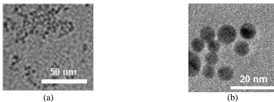
Fig. 1. Silicon (a) and gold (b) nanoparticles prepared by laser ablation.
