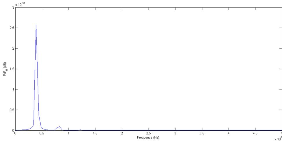
Fig. 4. Frequency domain of the SMI signal.
