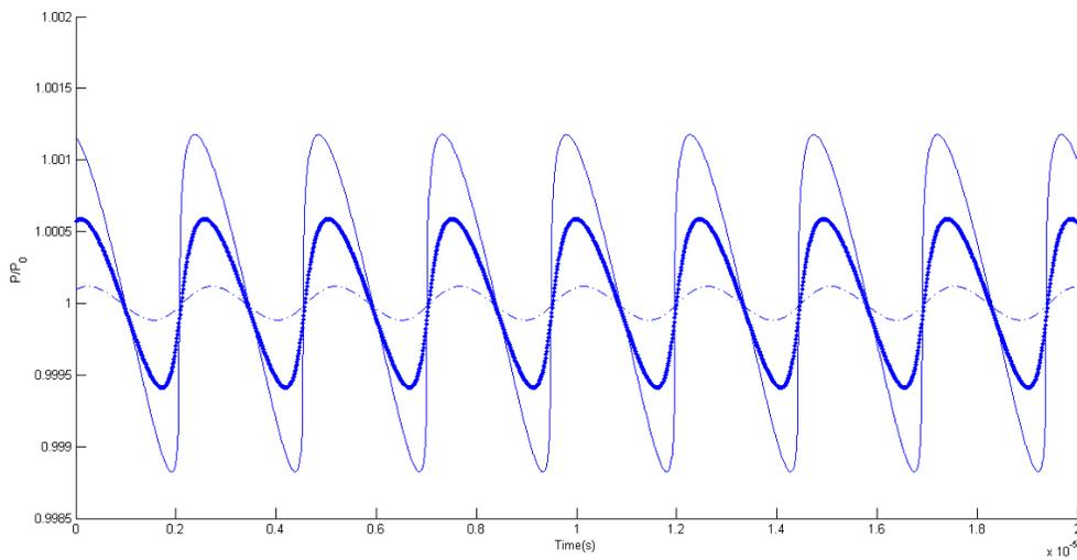
Fig. 5. SMI signals for values of  $C = 0.1$  (dotted line),  $C = 0.5$  (wide line) and  $C = 1$  (regular solid line).
